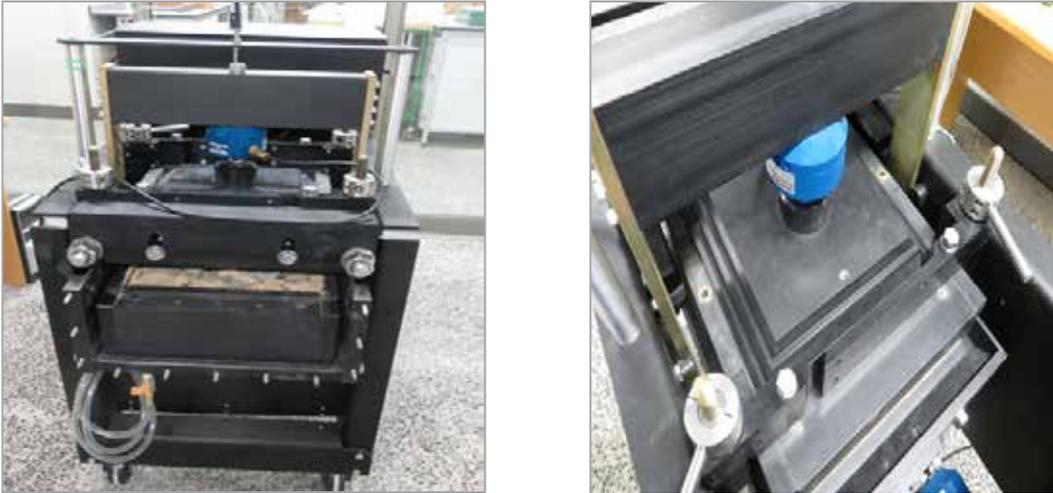
Figure 4: Compacted sample shear box placed in load frame for testing
