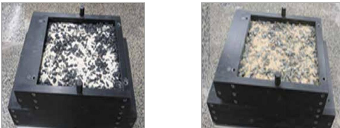
Figure 3: Specimen of compacted tyre shred-sand composites placed in the shear box
