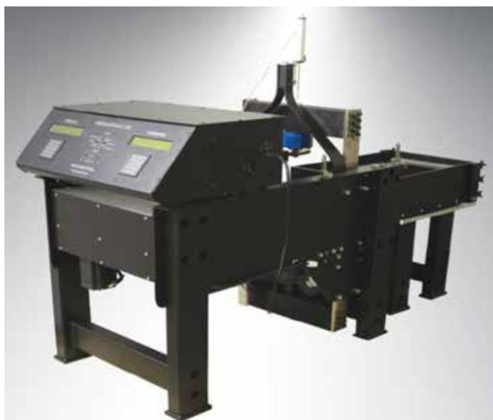
Figure 2: Automated large direct shear testing system (Geocomp ShearTrac-III Manual)
