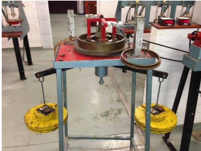
Figure 4. Ring Shear Apparatus.
