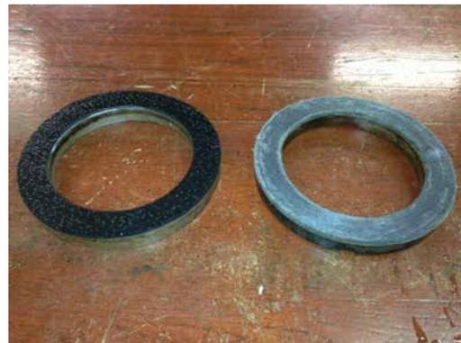
Figure 6. Geosynthetics after a ring shear test.
