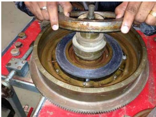
Figure 5. Close-up of ring shear apparatus.
