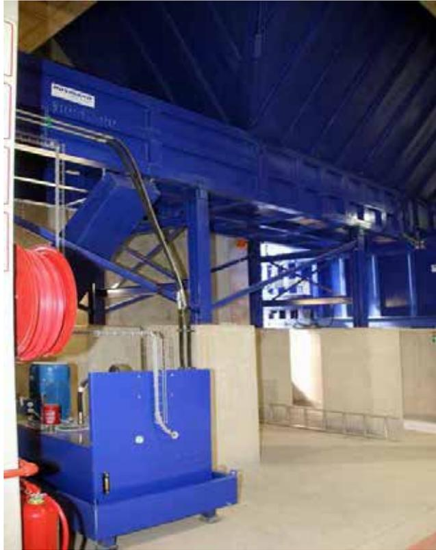
Figure 5: One of the three compactors (photo is of the one “side-pusher”). Waste is collected in the large hopper “basket-type” unit above and a ram then pushes the waste into a container.
