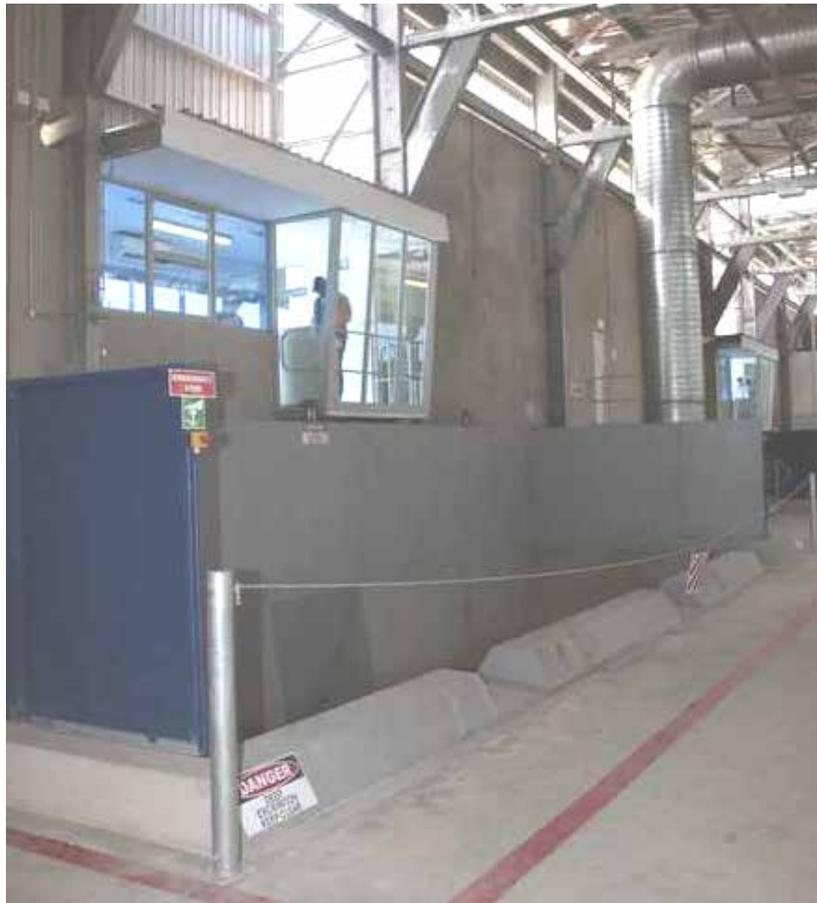
Figure 8: View of one control booth and the open chute. (Waste collection vehicles would reverse up to the open chute and offload waste into the unit.)
