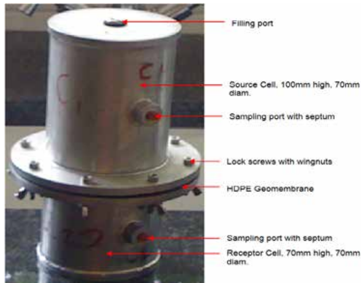
Figure 6. Diffusion Test Cells used in this study
