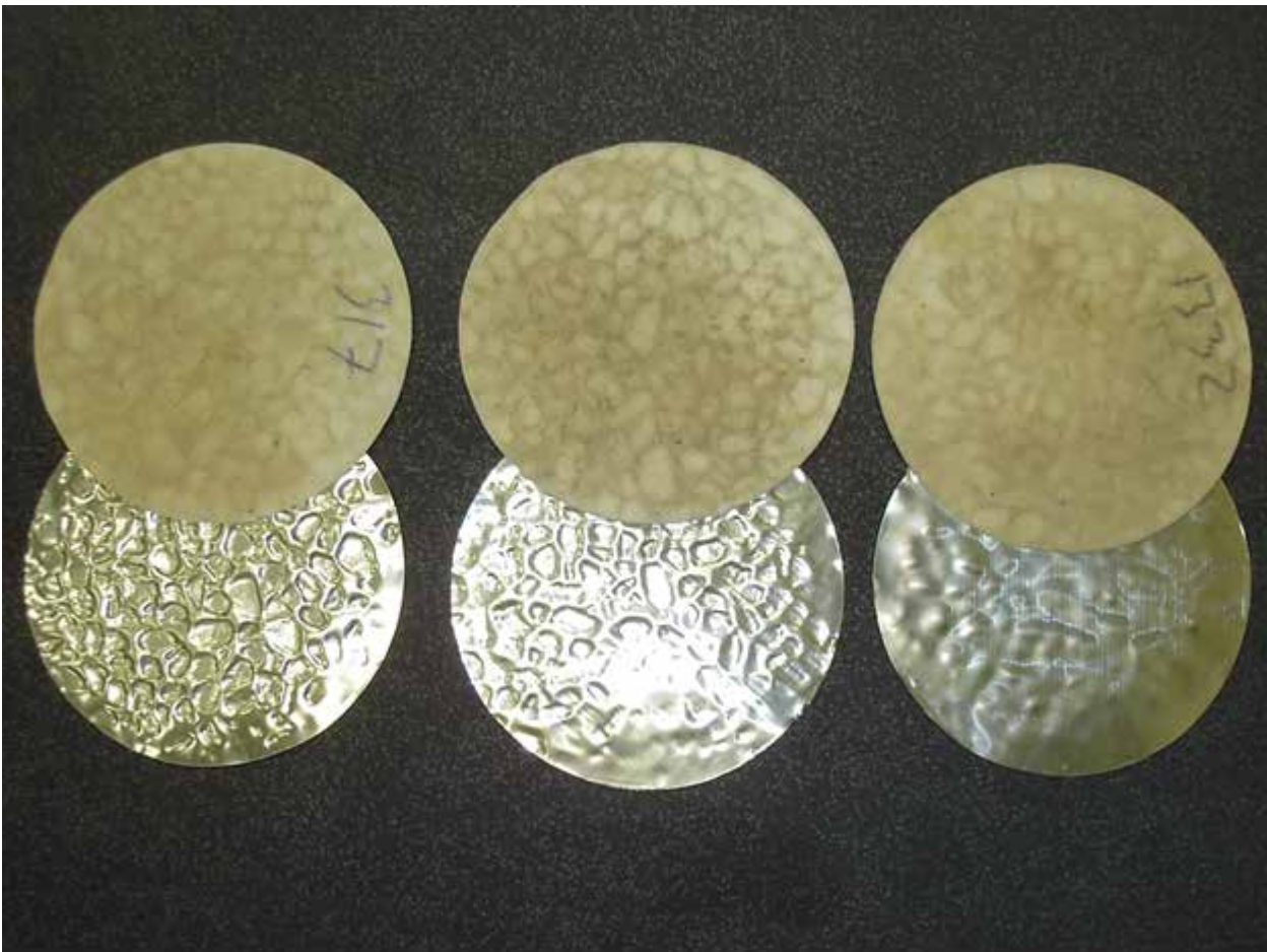
Figure 3. Plate bearing test using protection geotextiles with different mass per unit area on top of a 1.5 mm thick HDPE geomembrane at the same test conditions (NAUE GmbH & Co. KG)
