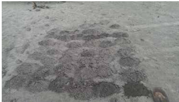
Figure 1 - Ash Samples from Borehole for Borehole Logging
