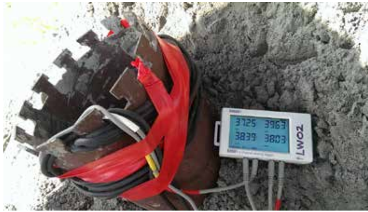
Figure 2 - Initial Temperature Readings from Borehole Test Station
