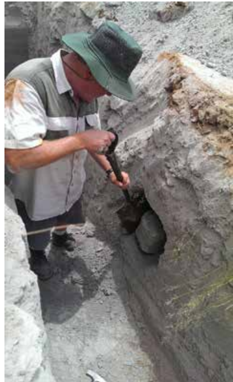
Figure 2 - Removing the undisturbed ash sample
