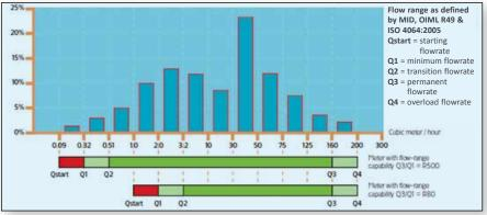
A meter with basic flow-range capability (R80) doesn't record the flow below 1 m3/h and is accurate only above 2 m<sup>3</sup>/h.
